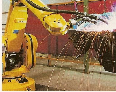
Metal fabrication is completed by a robotic welder. The robot's particular talent is repeated precision. Errors are eliminated.
