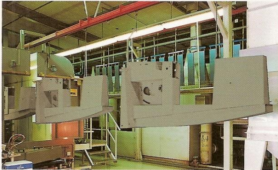
The powder coating unit with 12 nozzles delivers a quality finish so that your HOLZ-PRO professional machine will remain as new for years to come.
